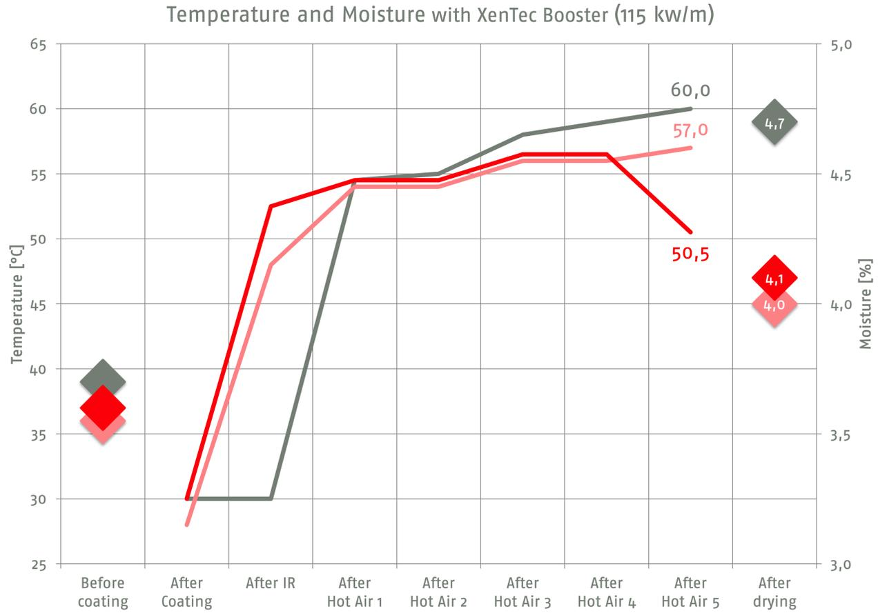
The booster at 73% power reduces the temperature by 9.5°C at reel with 3.5°C lower max. temperature as during radiation water is evaporated, using steam enthalpy for cooling down the surface.
