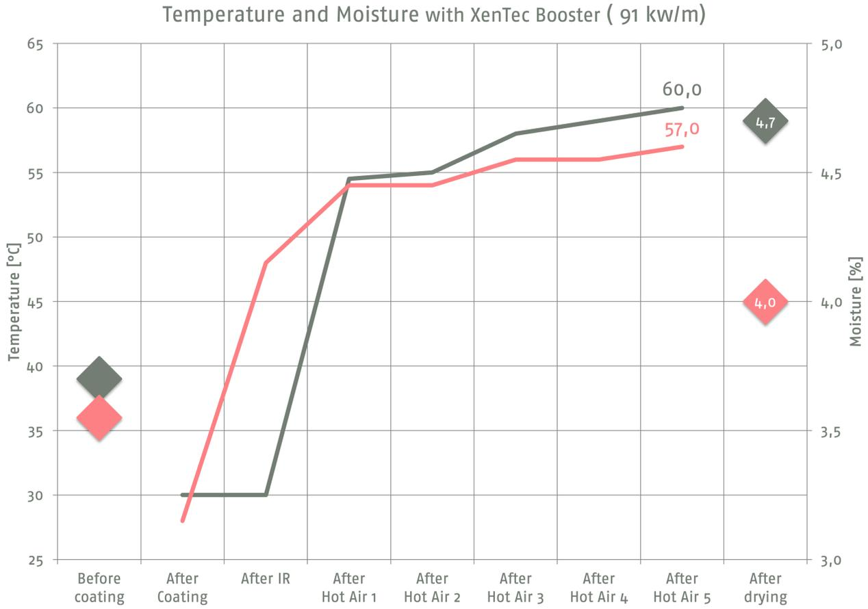
The booster at 57% power reduces the maximum temperature as during radiation water is evaporated, using steam enthalpy for cooling down the surface.
