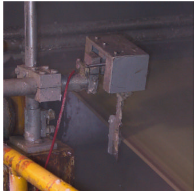
III. 1.: ElectroPalm in the felt of a crescent former with oscillation to avoid damage caused by edge trimming.
